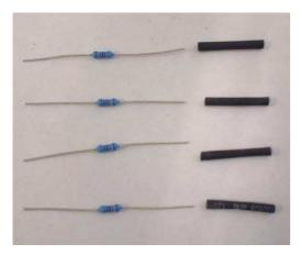
Cover one leg of each resistor with the shrink tubing, and shrink it on. Make sure some wire is exposed at each tip to allow soldering of the resistor. Also expose where the wire reaches the resistor, for soldering.
