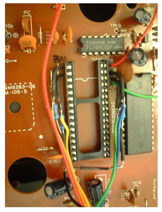
Bend over some corner socket pins on the track side while pushing the socket in place, so that the socket is held in place by itself.
