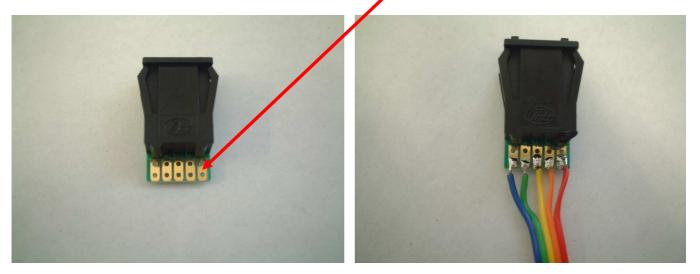
This cable is probably very excessively long when mounted in the DM100, but for now it is good to have it long until you decide where you want to mount the encoder switch. Just cut the cable when you decide and reconnect it to the encoder with a more convenient length when you're ready to mount it.
