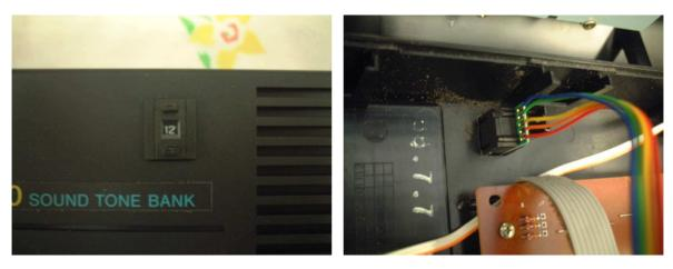
Re-solder the encoder wires.
