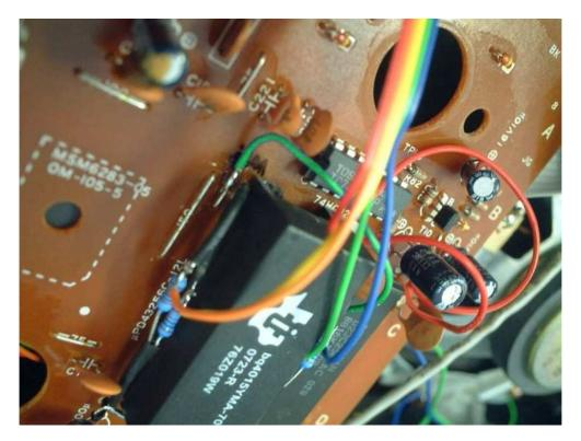
The bottom of the chip should be next to where the **black wire** is at the ends of the resistors.
