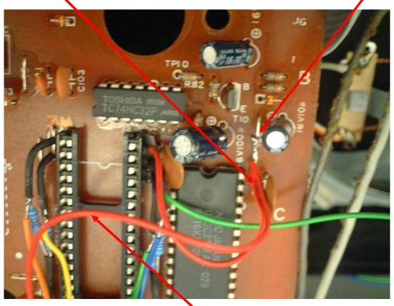
Solder the free end of the **red wire** that goes to the "C" terminal of the rotary encoder also to this same jumper. This is the power wire to the encoder. The silver wire jumper is a convenient **+5V power supply** point on the board.
