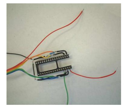
Solder the other ends of the orange, yellow, green, and blue wires to the terminals labeled 1, 2, 4 and 8 of the rotary encoder. Solder the red wire of this end to the terminal labeled "C" of the rotary encoder.
