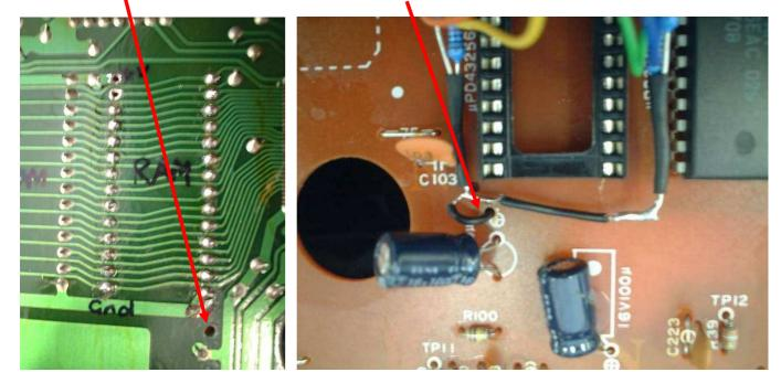
On the track side of the board, solder the other end of this **black wire** to this solder point on the circuit board:
