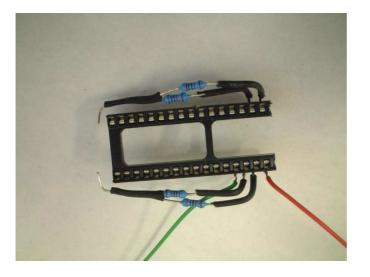
Solder the free ends of the resistors as show to each of the socket pins:
